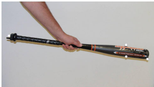
Fig. 12 Instrumented bat used for benchmarking study. Five reflective markers (four of which are visible in this image) were used with VICON motion analysis system to determine the velocity of the sweet spot. The knob-mounted IMU was used simultaneously to determine the velocity of the sweet spot
